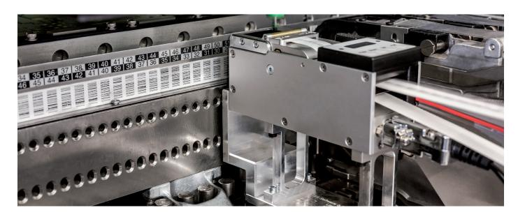
Quick. Easy. Reliable. That's the **ALF14 Label Feeder**. The hard-working, high-tech helper that adds efficiency to your product manufacturing. With a compact design, this device offers automated label feeding at an affordable price. It fits well with existing SMT lines, plus it offers improved traceability — especially when used with Brady materials: white polyimides, laser markable materials and polyimides masking film. And, the ALF14 helps out in other ways, too:
