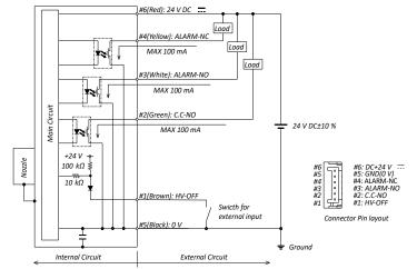
Note1: Use mechanical switch or photo coupler or relay for external input. If the grounding potential of external device to use for external input and the grounding potential of this product use are different, the external device used for external input should have an insulated on/off procedure for the 0 V line
