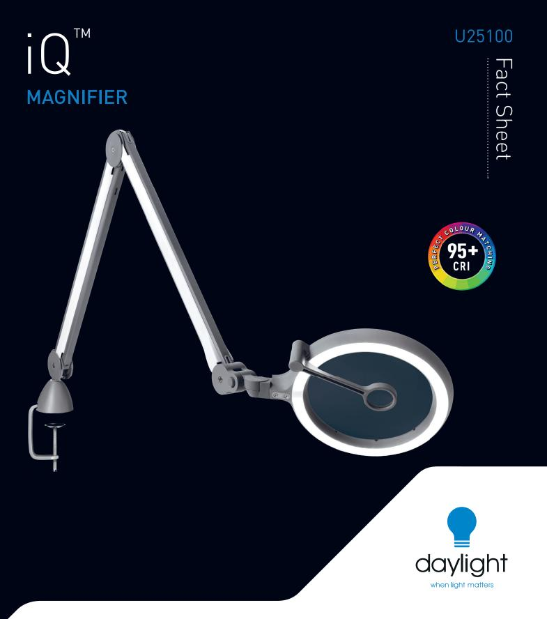
The iQ magnifier has a 7" lightweight acrylic lens offering a large field of view. The magnifying head moves freely and holds any position - maximising horizontal and vertical movements. The heavy-duty internally sprung arm provides good horizontal reach and will stay in place. A 12 diopters (4.0X) magnification lens mounted on a swing arm is also included. Lateral protections help you keep it clean. The magnifier is fitted with a removable lens protector.
