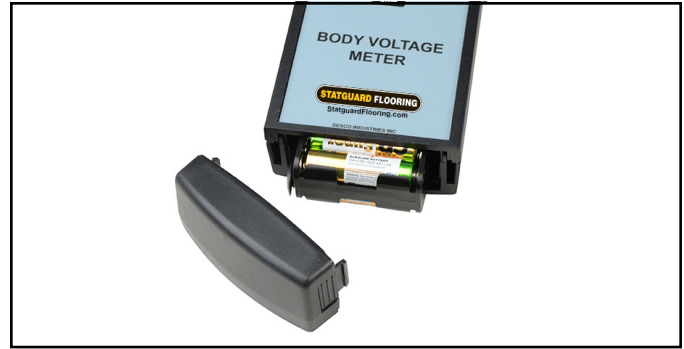
Figure 9. Replacing the Batteries on the Body Voltage Meter
