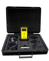
The measurements can be performed either with the built-in measurement electrodes on the underside of the instrument, with external probes such as the **SR400 Miniprobe** or the **SR820 Lightweight Travel Electrodes**. Performed measurements with external measuring electrode meet the requirements of ANSI/ESD STM4.1, ANSI/ESD STM7.1, ANSI/ESD STM2.1, ANSI/ESD STM12.1
