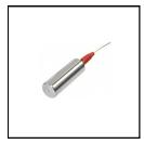
Designed to be used with resistance meters to evaluate ESD flooring according to ANSI ESD20.20. The probe is held in the hand while performing Walking Tests and other resistance measurements.
