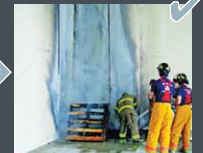
Result: Pass 25 ft. High Corner Test
