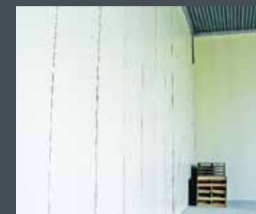
25 ft. high Corner Test Preparation
