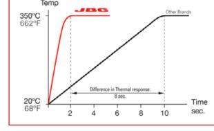
This rapid response is made possible because the handle and tweezer tools for the NASE and NANE workstations are designed with the heating element located close to the tool tip to ensure heat is delivered rapidly to where it is
