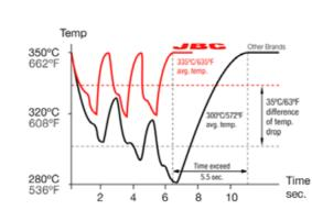
recover between connections, resulting in poor quality coldsoldered connections. To compensate for this an operator will often run a conventional tip at a higher temperature. This can shorten the tip's life and may even damage the PCB or the component being soldered - see graph.
