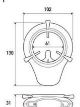
Double-row ring lights provides high-brightness — twice that of other ring lights! The short vertical LED illuminates the sample from a perpendicular position.
