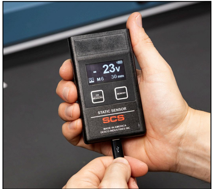
Figure 8. Connecting the USB-C cable to the Static Sensor
