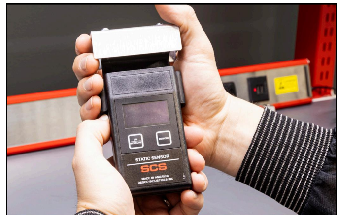
Figure 13. Sliding the Conductive Plate onto the Static Sensor
