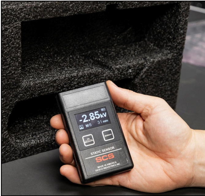
Figure 7. Using the Static Sensor to measure foam
