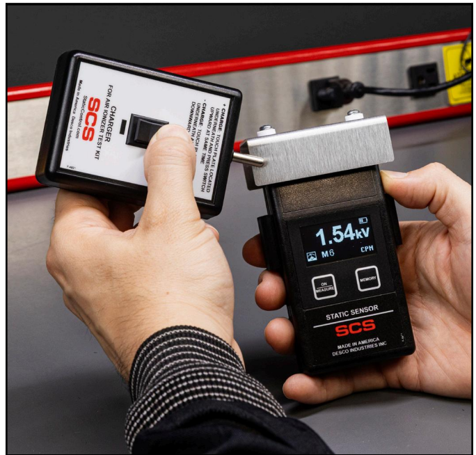
Figure 15. Using the Charger to apply a positive charge onto the Conductive Plate
