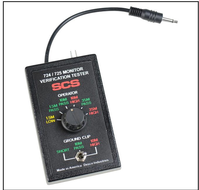
Figure 12. SCS 770065 Verification Tester
