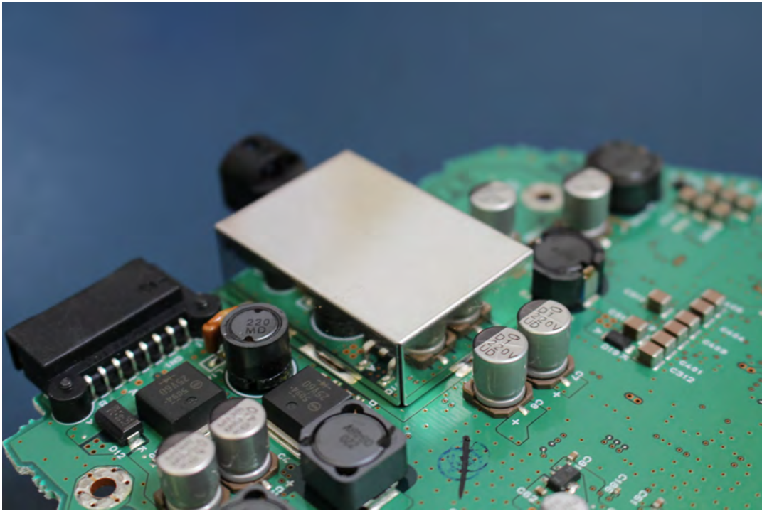
Figure 6. RF shielding soldered to PCB.
